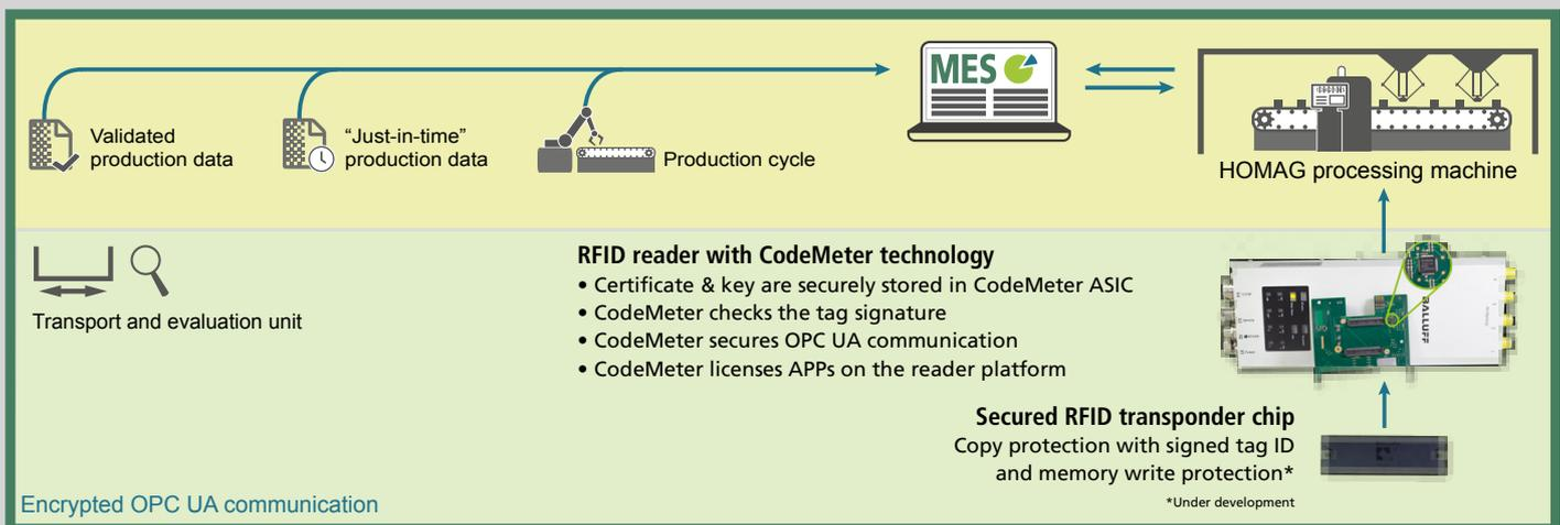
full licensing capabilities and secure updates, making it possible to upscale the reader's functionality in the field. At the same time, all communication can be encrypted end-to-end, putting an end to the most easily disrupted part of the communication process, i.e. the radio transmission between tag and reader.
