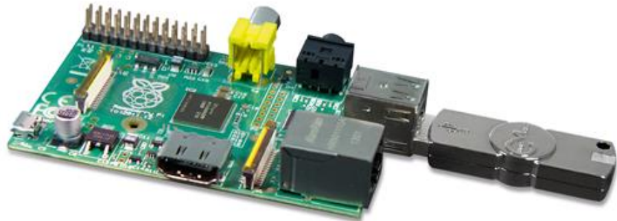
Pic.: Raspberry Pi with CmStick, the USB dongle for software protection, plugged in
