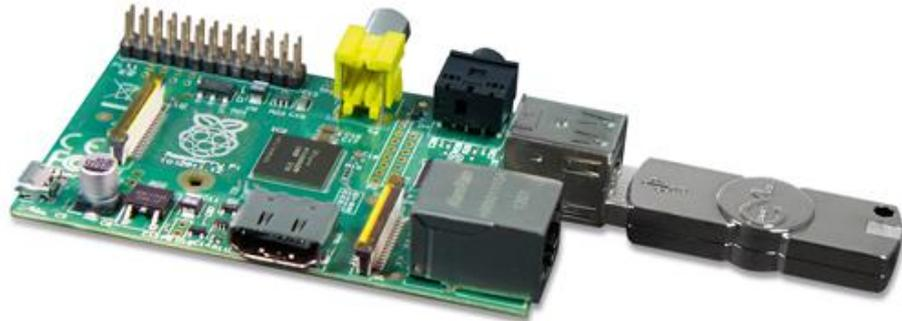
Picture: Raspberry Pi with the USB dongle CmStick connected.
